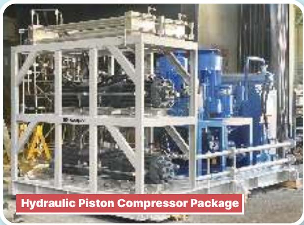
Hydraulic Piston Compressor Package
